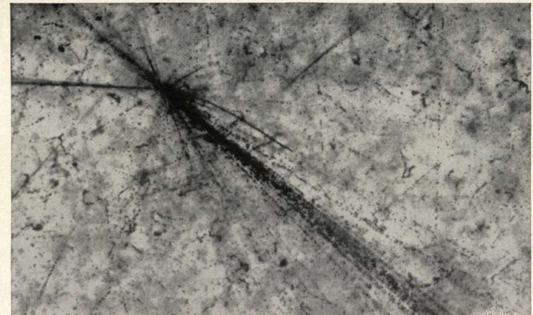
COSMIC PARTICLE caused this tiny explosion revealed by a photomicrograph of a photographic emulsion especially prepared to record nuclear events. An exceptionally energetic helium nucleus struck a heavier nucleus in the emulsion, giving rise to the jet of mesons going off to the lower right. These photographs were provided by Herman Yagoda of the National Institutes of Health.
